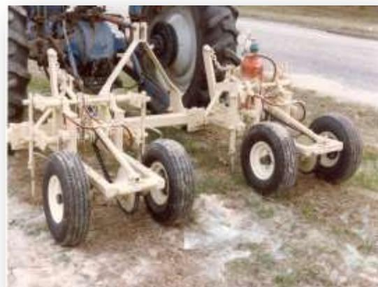
'Sewing Machine' Punch Injector for use in Lawns, Gardens, Highway Rights-of-Ways, etc.
